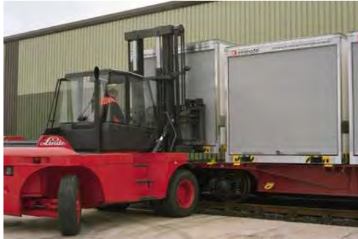
Figure 16: Smaller CT load units in UK
